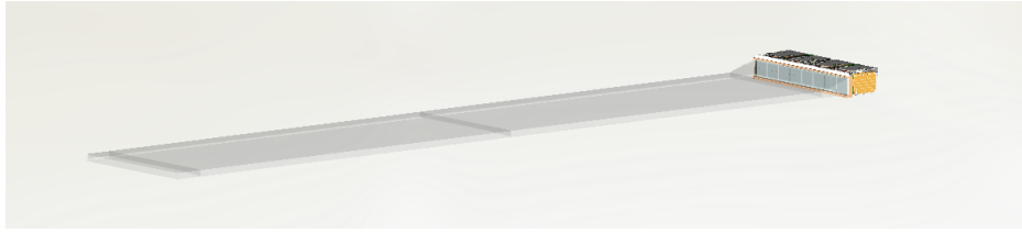
Figure 2.21.: An iTOP module with quartz, MCP-PMTs, and electronics, no QBB
