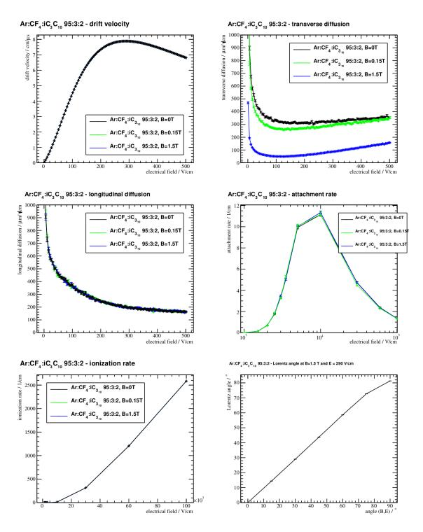
Figure 8.2: MAGBOLTZ simulation for optimal working point of electrical field for various parameters [37]. Maximal drift velocity achieved at  $E_{\rm D} = 289\,{\rm V\,cm}^{-1}$
