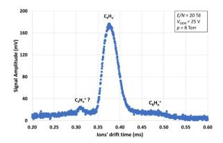
Figure 10.10: Typical drift spectrum for ions from the T2K gas mixture at p = 8 Torr [44].
