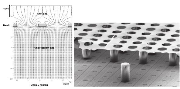
(a) Electrical field lines in a Micromegas [26]
