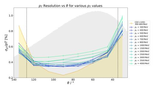
Figure 12.11:  $p_T$  resolution vs.  $\theta$  with individual curves for  $p_T$ . Average for CDC+VXD for  $p_T$  below 900 MeV is also shown. Effect of MS is visible for the CDC, but does not have large impact on the TPC. More details in the text. The gray histogram shows the  $\theta$  distribution of stable charged particles from  $\Upsilon(4S)$  events.
