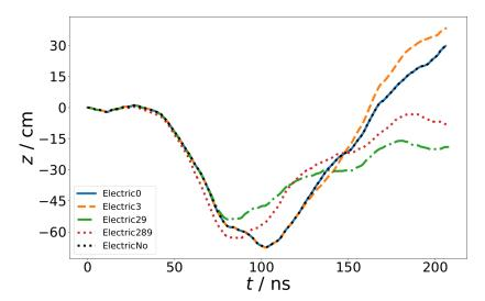
Figure 11.5: *z* vs. *t* for the same muon using different electrical field strengths. Entry "ElectricNo" indicates that the simulation was reversed to version without any implementation of the electric field. The effect of particles turning around is clearly independent of the electric field implementation.
