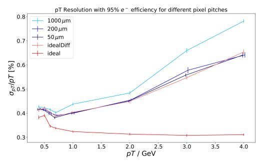
Figure 12.2:  $p_T$  resolution for varying pixel pitches and fixed electron efficiency compared to the *ideal* and *idealDiff* scenarios. The data points are slightly shifted with respect to the true  $p_T$  value for visualization purposes.
