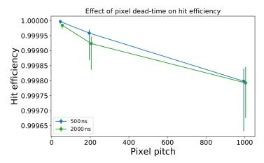
Figure 10.13: Hit efficiency for  $\Upsilon(4S)$  hits in the TPC volume including effects from pixel dead-time. For visualization the data points are slightly shifted in the *x*-axis.
