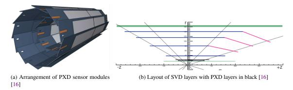
Figure 5.3: Design of the vertex detectors, PXD and SVD
