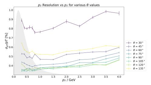
Figure 12.10:  $p_T$  resolution vs.  $p_T$  with individual curves for  $\theta$ . Worst resolution is achieved for muons which exit through endcaps. Rise in  $p_T$  resolution for large  $p_T$  independent of  $\theta$ . Therefore, it is likely that the lever arm dominates the position measurement term in the  $p_T$  resolution. The gray histogram shows the  $p_T$  distribution of stable charged particles from  $\Upsilon(4S)$  events for  $17^\circ \le \theta \le 150^\circ$ .
