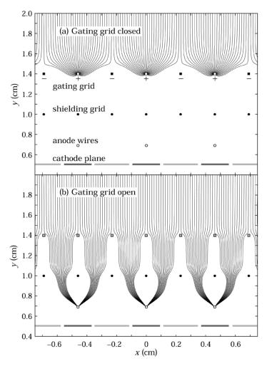
Figure 6.2: Electric field lines for closed and open wire gate [23]
