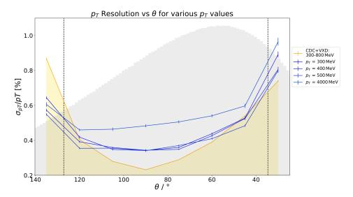
Figure 12.13:  $p_T$  resolution vs.  $\theta$  with curves for low  $p_T$  values. Scattering effect becomes more dominant for low  $p_T$  particles.
