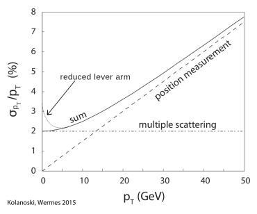
Figure 4.2: Contributions to the  $p_T$  resolution [3]. Multiple scattering contributes a constant term, while the position measurement adds a rise for  $p_T$ . Additional contribution from reduced lever arm at very low  $p_T$
