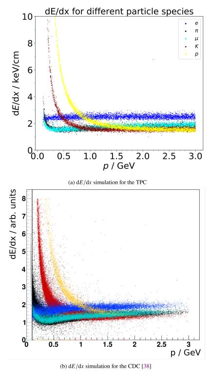
Figure 9.1: dE/dx from simulation for the TPC and CDC. Low  $p_T$  part which does not reach the TPC is low-lighted in the CDC plot.
