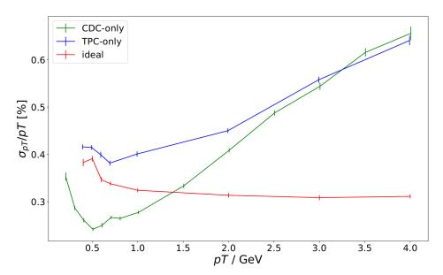
Figure 12.5: Comparison of  $p_T$  resolution for TPC-only with CDC-only. The CDC has a far better resolution at low  $p_T$ , mainly due to a constant multiple scattering term. They have a similar value at large  $p_T$ . Effect of diffusion on the position measurement can be seen by comparing to the *ideal* curve.
