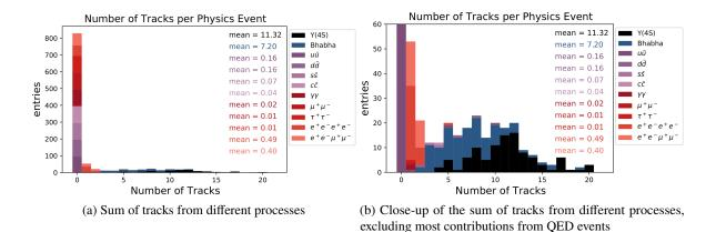
Figure 10.4: Sum of tracks in triggered TPC volume for all physics processes in Table 10.1. Mostly no tracks from QED or  $q\bar{q}$  events in the TPC, but large contribution from Bhabha scattering events.
