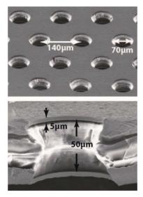
(a) Image of a GEM from a scanning tunneling microscope (above), enhanced cross section of a hole (below) [3]
