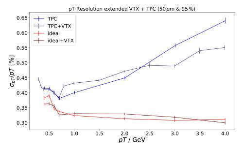
Figure 12.6:  $p_T$  resolution for TPC+VTX scenario compared to TPC-only case. VTX has a slight negative impact for low  $p_T$  particles, but improves resolution for higher  $p_T$ . The curves for *ideal* and *ideal* +VTX are consistent with each other. The VTX does not improve on the *ideal* case, since without diffusion the lever arm contribution lies outside of the regarded momentum range.
