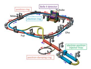
Figure 5.1: Schematic design of the SuperKEKB accelerator [10]
