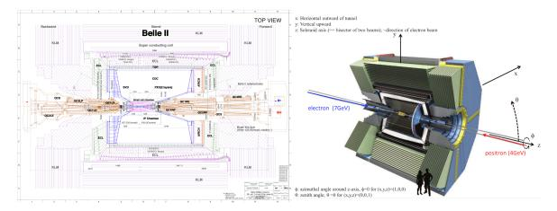
Figure 5.2: Left: technical drawing of Belle II detector design with focusing quadrupoles [14] Right: Coordinate system of Belle II detector. The interaction point marks the origin of this coordinate system. [15]
