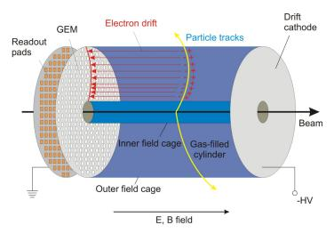
Figure 6.1: Working principle of a TPC with electrons from ionization due to the charged particle drifting towards the readout region [22]
