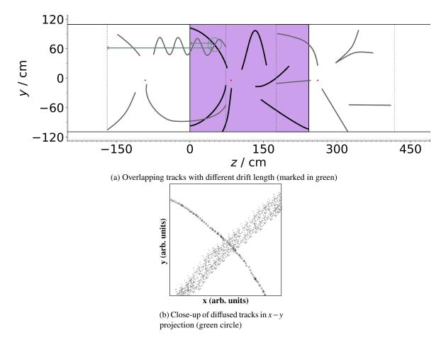
Figure 10.6: Illustration of the effect of diffusion on overlapping tracks with different drift lengths. The gray track belongs to an earlier event and has therefore a large drift length. The black track belongs to the triggered event and has a short drift length. Based on the diffusion one can distinguish the tracks even though they have the same reconstructed z coordinate (provided that drift time measurement starts with the trigger for the central (black) event).
