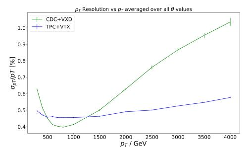
Figure 12.8:  $p_T$  resolution vs  $p_T$  for TPC+VTX compared to CDC+VXD averaged over all  $\theta$  values. The shape of the curves is largely the same with a few deviations for the  $p_T$  resolution
