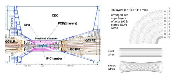
Figure 5.4: Design and wire configuration of the CDC [17]. The skew of the stereo wire configuration is exaggerated.
