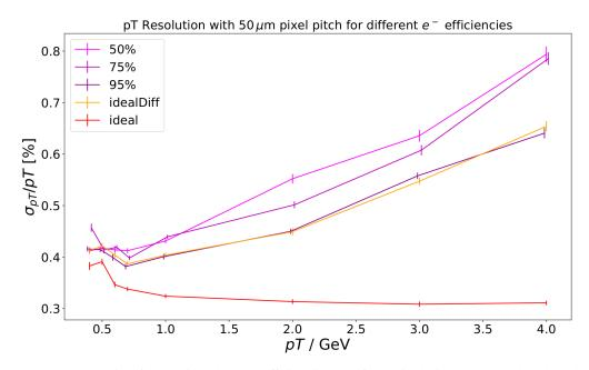
Figure 12.3:  $p_T$  resolution for varying electron efficiencies and fixed pixel pitch compared to the *ideal* and *idealDiff* scenarios. Again, the *ideal* case has the best resolution. With decreasing electron efficiency the deterioration in the  $p_T$  resolution becomes visible.
