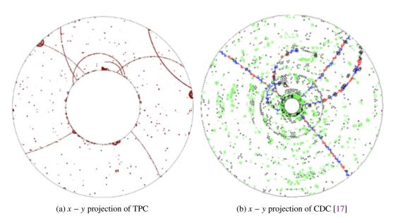
Figure 12.4: Showcase of the shorter lever arm of the TPC leading to worse  $p_T$  resolution. Inner region of TPC to be filled with VTX.
