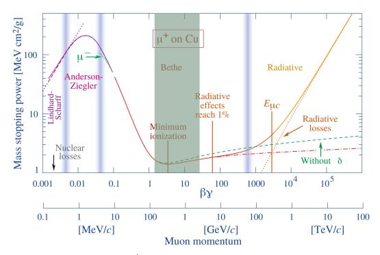
Figure 3.1: Mass stopping power for  $\mu^+$  in copper [2]. Particles are considered to be minimally ionizing at  $\beta\gamma \geq 3$  up to  $\beta\gamma \sim 1000$ . Highlighted in green is the expected momentum range for pions in Belle II which are the most common charged particle from  $\Upsilon(4S)$  events [4].
