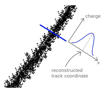
Figure 12.12: Reconstruction of a track position using the charge density perpendicular
