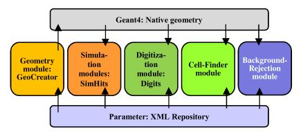
Figure 8.1: Chain of a basf2 job with time going from left to right. Geometry parameters are taken from a xml repository and used for the simulation. [33]
