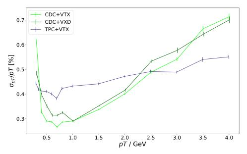
Figure 12.7:  $p_T$  resolution for TPC+VTX scenario compared to CDC+VXD and CDC+VTX. The extension of the lever arm due to the VTX causes a better  $p_T$  resolution for the TPC at high  $p_T$ .
