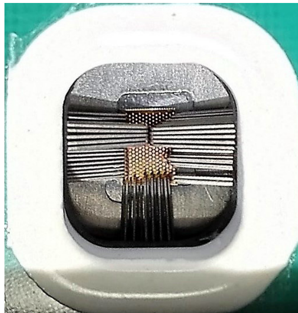
Figure 4.29: Top view of the needle spider inside the cut-out of the PCB. A DHP v1.1 is aligned and connected.
