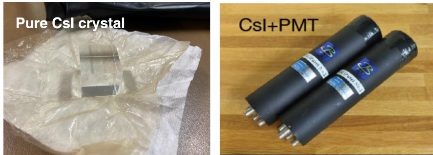
Figure 3.3: Pure CsI crystal and PMT attached with CsI
