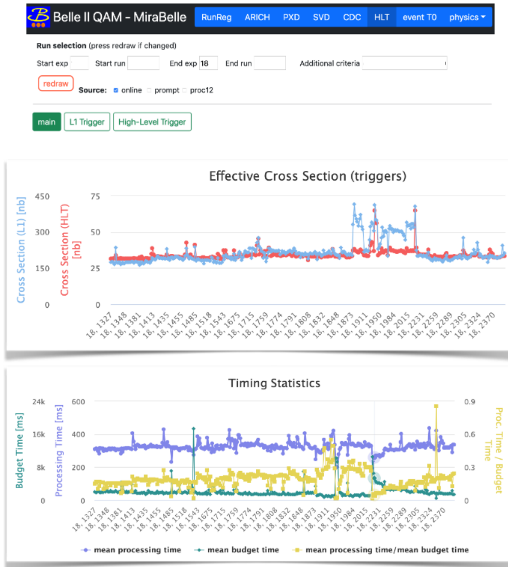
FIGURE 2.13: HLT related plots on Mirabelle monitoring system for certain runs in Experiment 18. The top plot shows the effective cross-section, while the bottom plot shows the average processing time per event.
