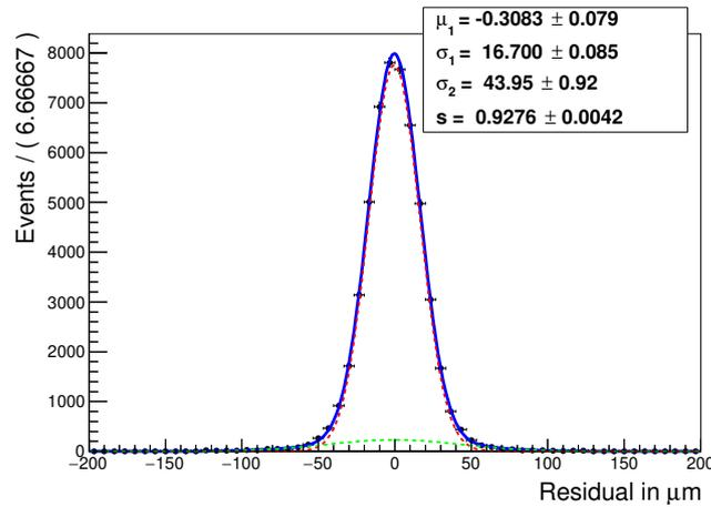
**Figure 3:** Residual distribution for the 6<sup>th</sup> layer 3<sup>rd</sup> sensor U-side with cluster size one.
