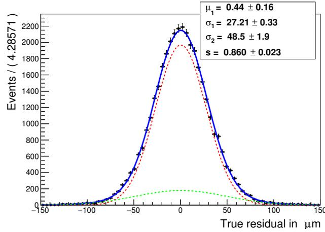
**Figure 4:** True Residual distribution for the 6<sup>th</sup> layer 3<sup>rd</sup> sensor V-side with cluster size one.
