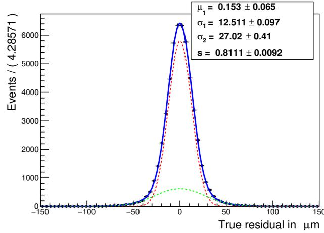
**Figure 2:** True residual distribution for the 6<sup>th</sup> layer 3<sup>rd</sup> sensor U-side with cluster size one.
