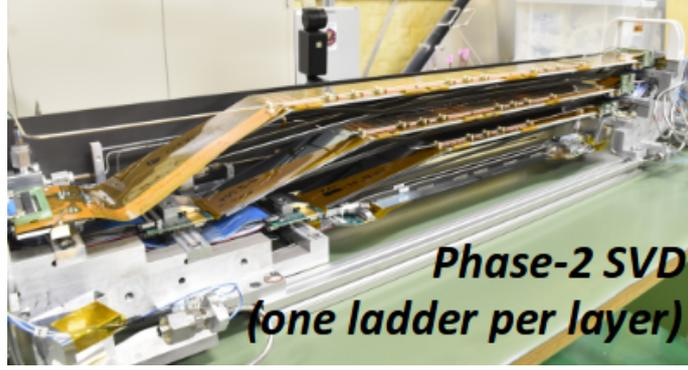
**Figure 1:** Layout of the Phase-2 SVD with one ladder per layer. Going from outward to inward, one can see layer-6, 5 and 4 (layer-3 and PXD layers are barely visible).
