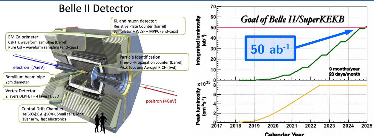
Innermost layer of the vertex detector is 2 times closer to the IP w.r.t. Belle Great performances expected in the reconstruction of final states with neutrals and missing energy
