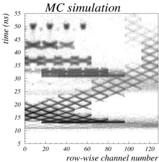
Perpendicular impact of a narrow 2.1 GeV/c positron beam
