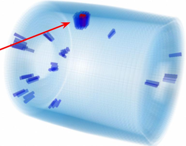
Simulated calorimeter event with reducible background
