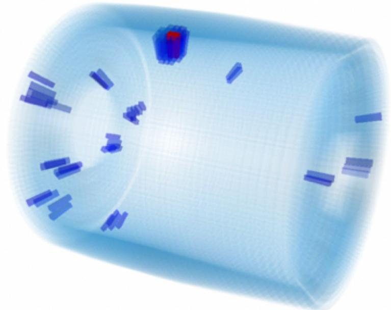
Simulated calorimeter event with reducible background
