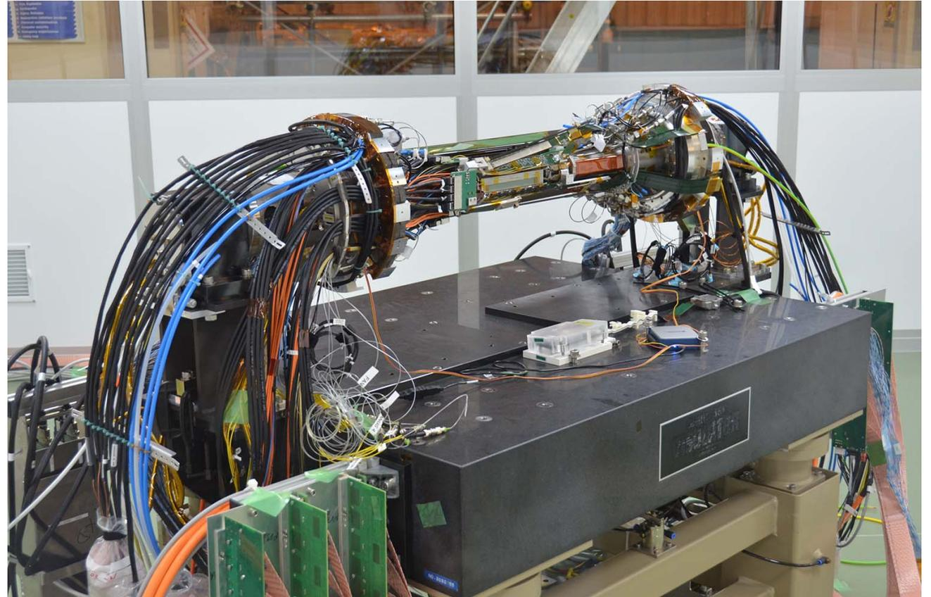
BEAST II detector after assembly on the central beam pipe
