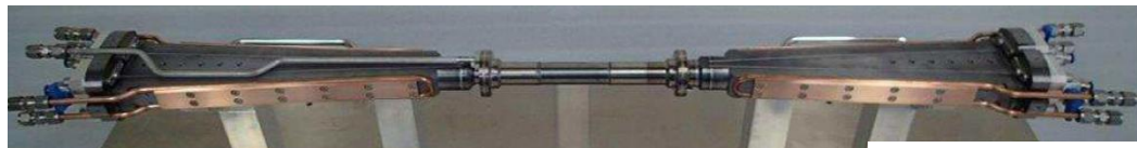
IP Beam pipe
