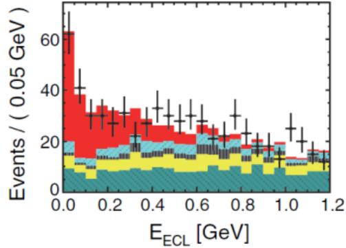
$E_{\text{ECL}}$  remaining energy in the calorimeter
