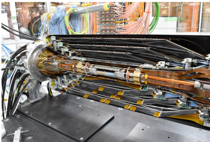
The complex superconducting final focus is partially visible here (before closing the endcap).
