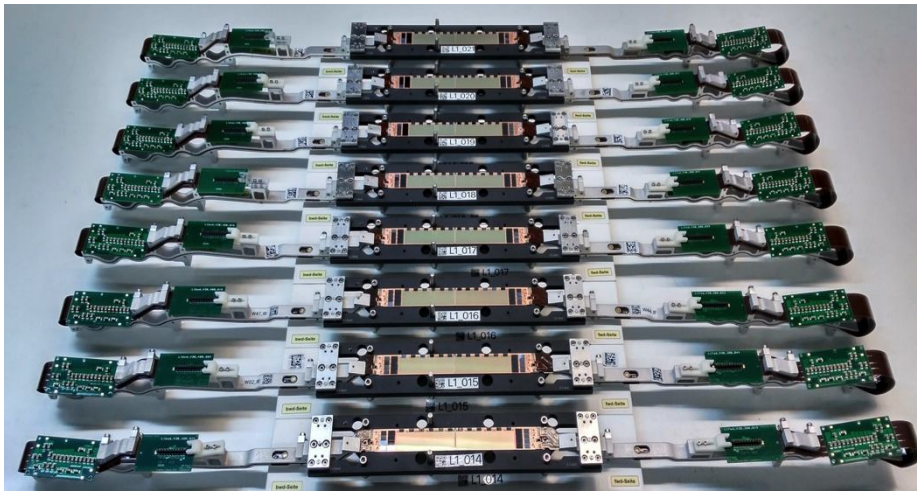
PXD layer 1 ladders, Feb 2018
