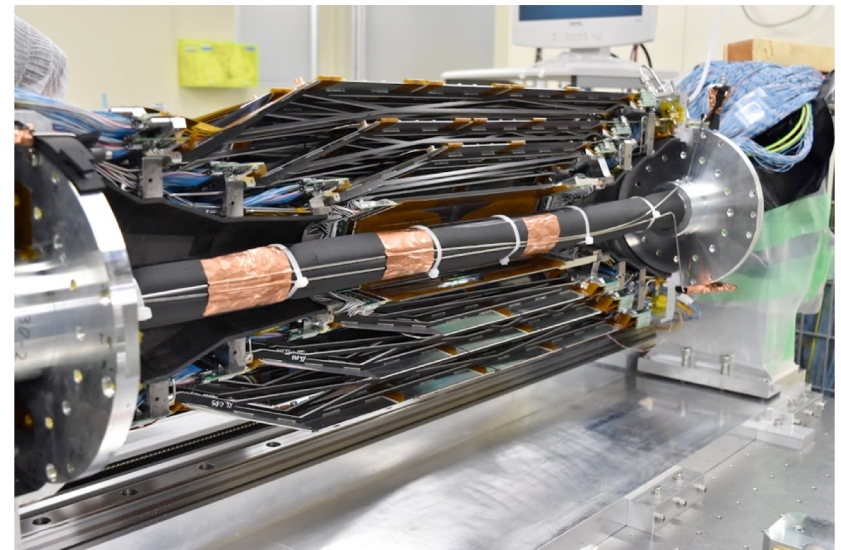
Completion of the first SVD clam-shell in Jan 2018.
