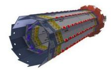
Precise silicon vertex detectors help to pin point the decay vertex of the particles like the D<sup>0</sup> and D<sup>+</sup>
