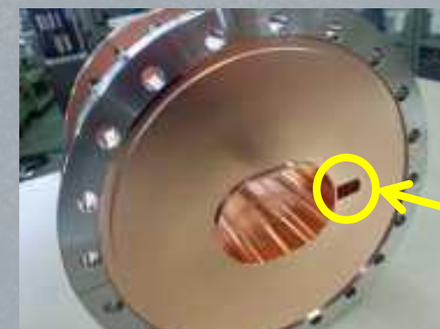
Beam channel for injection
